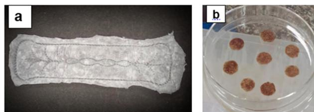
**Figure 3:** a) Cellulose matrix of sanitary napkin (Stayfree), b) discs of cellulose matrix incorporated with nanocomposite
