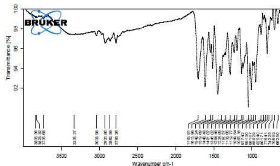
**Fig. 3: FTIR of ofloxacin with polymers
