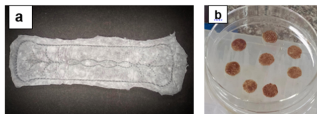
Figure 3: a) Cellulose matrix of sanitary napkin (Stayfree), b) discs of cellulose matrix incorporated with nanocomposite
